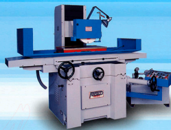
PFG-0408DAH 400 x 800 mm. Table Surface Hydraulic Longitudinal Feed Auto Cross Feed Manual Vertical Feed Table Longitudinal Travel is Controlled by Sensor and Solenoid Valve Continuous Lubrication.
