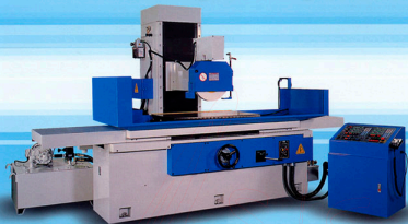
PFG-60100AHR 600 x 1,000 mm. Table Surface With Type AD5 Auto Down Feed Control and NC Parallel Dresser (Option) Hydraulic Longitudinal Feed Auto Cross Feed Vertical Feed is Driven by AC servomotor
